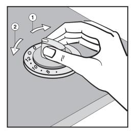
A burner with the symbol ◎ is activated by turning the respective control knob clockwise, ①, to the desired setting. It is turned off by turning the knob counterclockwise, ②, to "0".
